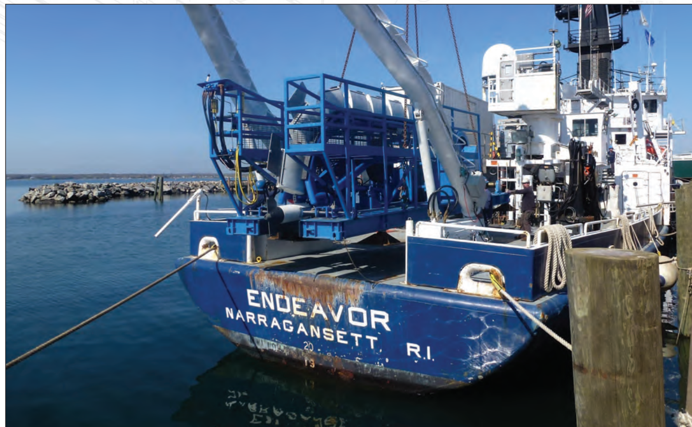
Mobilization of a vertical array launch & recovery system
