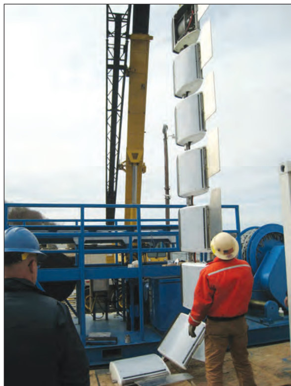
Eight element vertical towed array loaded into handling system
