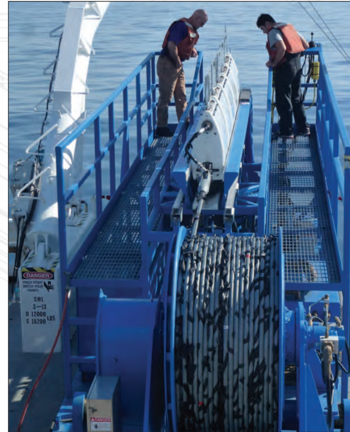
Dockside deployment of vertical towed array
